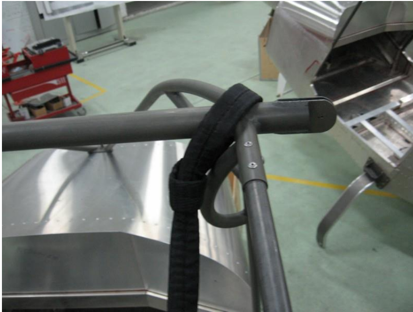
Picture 8.9a: Parachute ropes-front connection points
