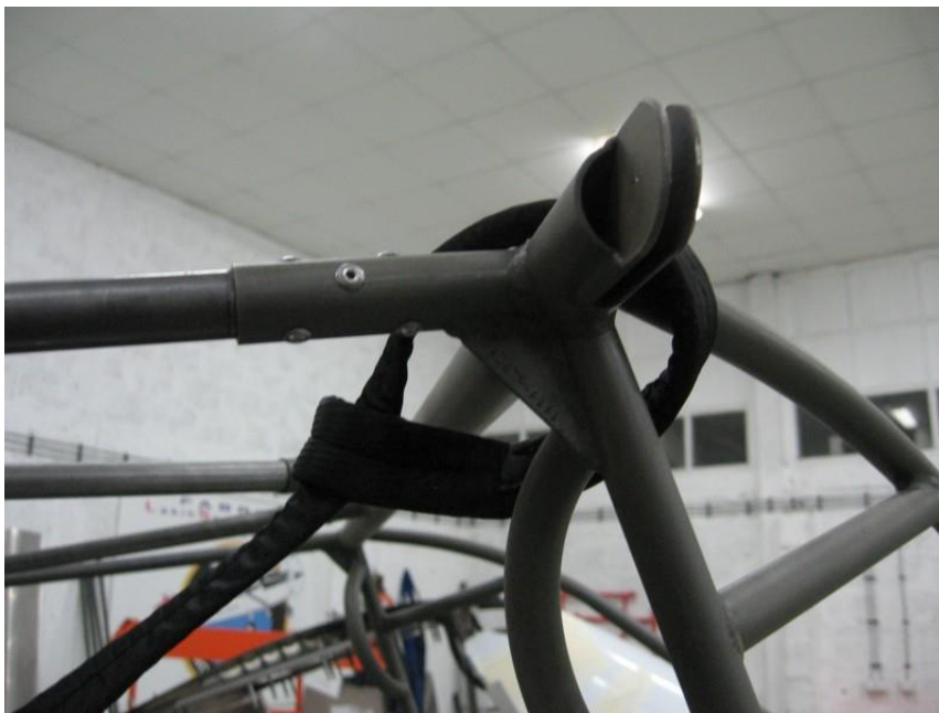
Picture 8.9b: Parachute ropes-front connection points
