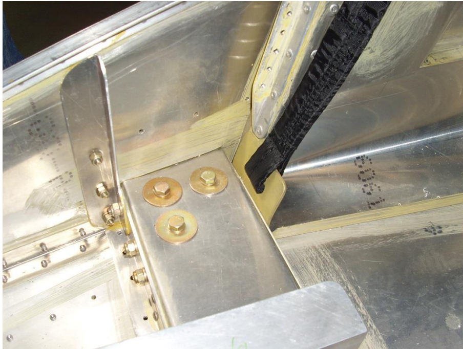
Picture 8.10a: Parachute ropes-rear connection point
