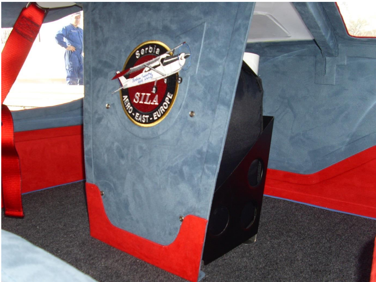
Picture 8.1: Position of the parachute on the SILA 450 C aircraft
