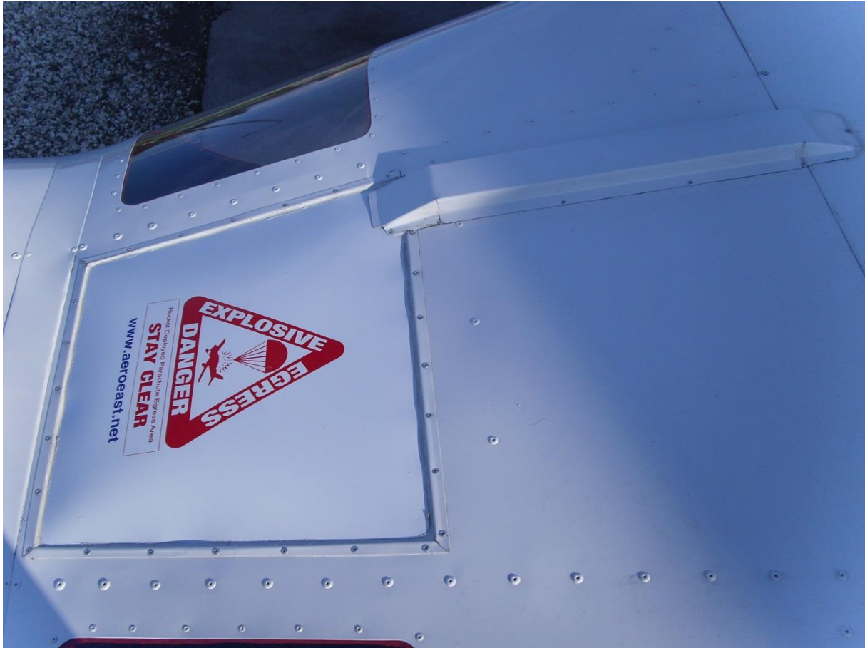
Picture 8.5b: Location of the parachute hole on the SILA 450 C aircraft
