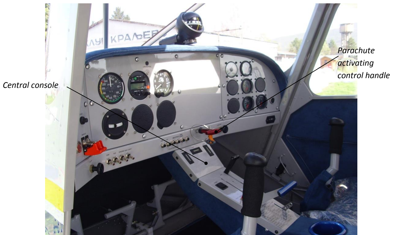
Picture 8.13: Parachute activating control handle
